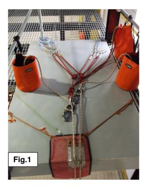
Rig the descent rope and back up through a descender attached to the main anchor points.
