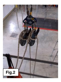
2. Ropes can be rigged from above the worksite but ensure they can be reached easily if required. **Fig.2**
