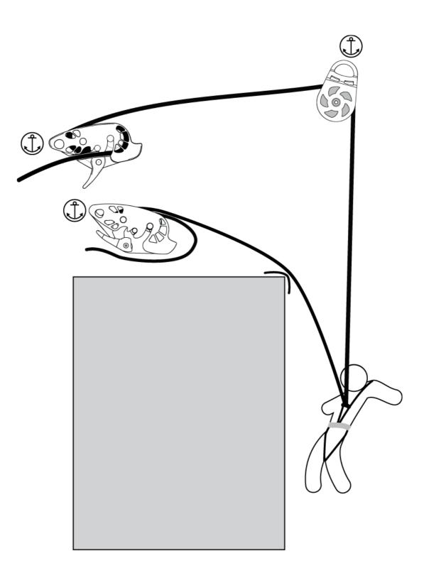
Example of rigging for rescue in rope access
