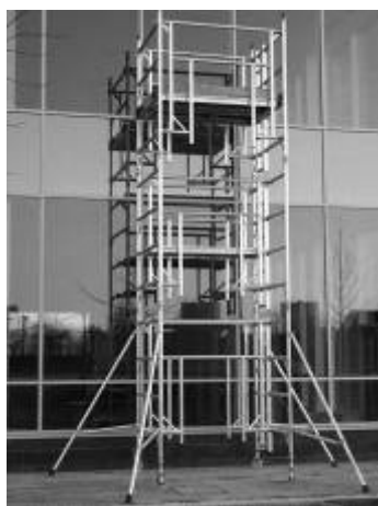
Primary support: Platform Fall protection: Guardrails
