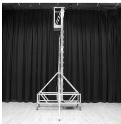
Primary support: Tallescope Fall protection: Basket/guardrail
