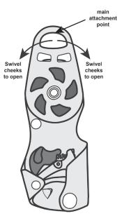
For use only with 10.5mm to 11.0mm diameter low-stretch rope.
