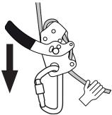
Pull this section of loop to move device towards anchor
