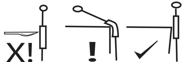
**The Square** rope protector, is a heavy duty, double layer construction pad, designed to be fastened directly to the structure or rigging and is ideal for protecting multiple ropes in rope access and rescue systems. The protector should be positioned and secured in such a way that the ropes are protected from contact with the abrasive surface using the cord supplied and prefitted eyelets.
